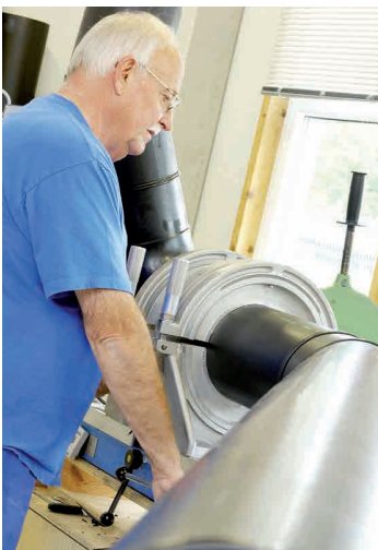
Pre-assembly of the pressure pipe system
